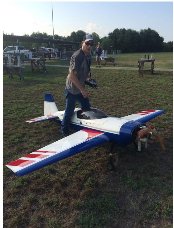
Brady is preparing to run up the engine on his big (40%!) Extra from DR Hobbies. All composite 118" wingspan, 180cc twin, 40lbs. Photos by Frank Sodek
