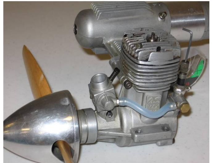
Used O.S. .61FX w/ muffler, spinner and propeller.
